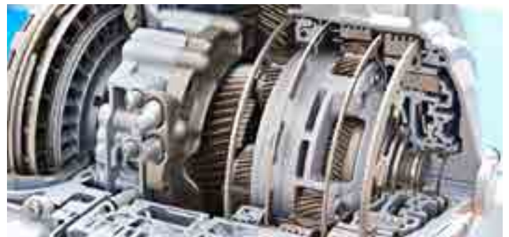
Automatic transmission reveal.
